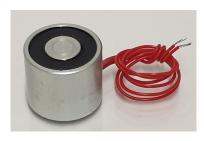
This magnet exerts a holding force of approximately **12 Kgf** perpendicular to any steel plate (see accessories) with which it is in contact, assuming nominal voltage, and coil at working temperature rise of 60°C in an ambient of 20°C.
