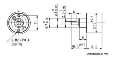
Note) Dimension marked  $\times$  is measured with shaft pushed against gearhead.
